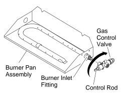
Figure 11 - Installing Gas Control Valve
